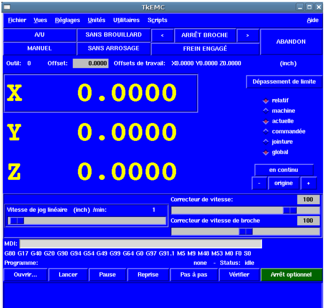
Figura 2.7: TkLinuxCNC graphical interface
